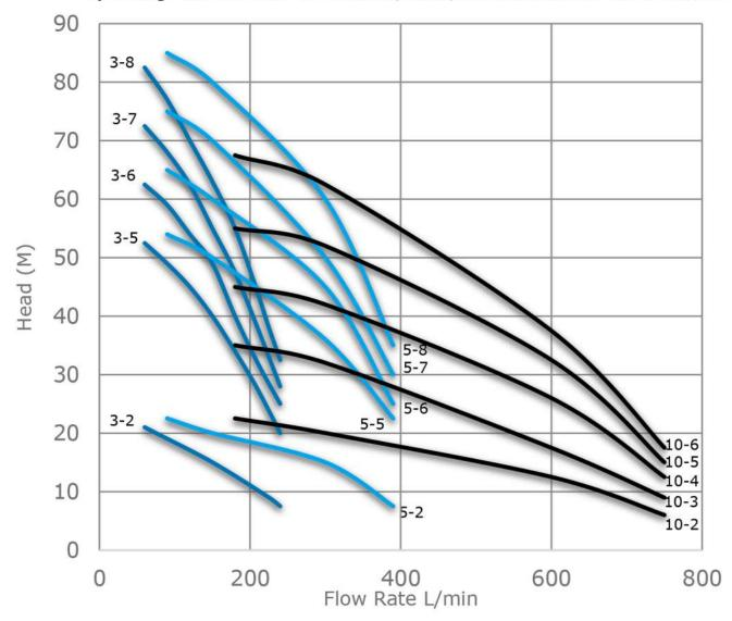
All systems set at mid curve efficiency during first activation on wet test using the RS variable speed inverter at closed valve up to max pressure. The performance curves are based on kinematic viscosity values = 1/mm2/s and density equivalent to 1000kg/m3.
