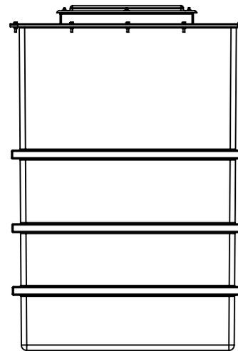
40mm Encapsulated RHS Steel Bracings
