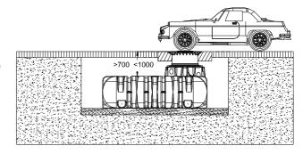
Coverage heights with cast telescopic dome shaft with cast iron lid or Begu (with cover class B respectively D - to be provided at construction site). Maximum load of the area used by passenger cars 3,5 to.
