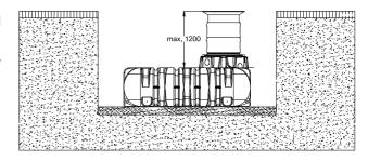
Coverage heights with cast telescopic dome shaft (class B) in areas used by passenger cars.
