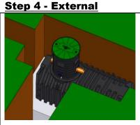
Backfill/Ballast In Stages To **Support Tank**
