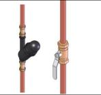
**Connect Inline Filter & Shut** Off Valve
