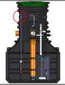
**Secure Mains Top Up Float** to bracket with cable tie
