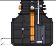
Mains Top Up Float to be positioned 150mm from base
