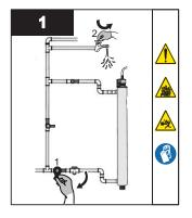
Close main water supply to the UV System, and then open a tap downstream of the UV System to release pressure.
