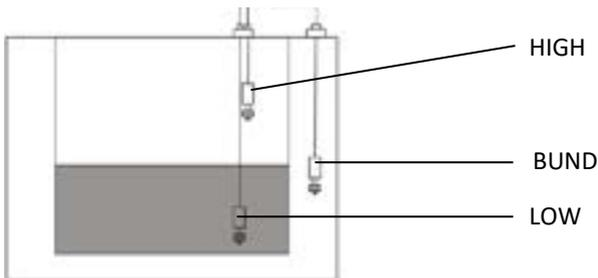
The probe wired to the **HIGH** connection is positioned at the topmost part of the tank and is used to alert that an overfill has occurred. The probe wired to the **LOW** connection should be positioned near the bottom of the tank to indicate a low-level. The **BUND** probe is placed between the two tank 'skins' and is used to quickly alert of any leaks.
