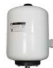
EXPANSION VESSEL 18L vessel on 250L cylinders 24L vessel on 300L cylinders 35L vessel on 400 & 500L cylinders
