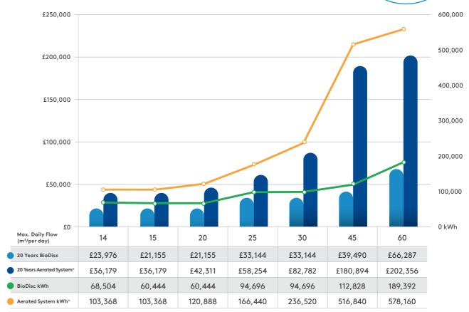
\*Based on Klargester BioFicient Aerated System
