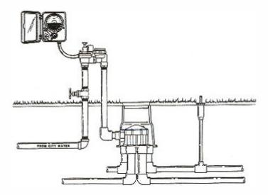
For high flow city water supplied installations using and in-line valve, ensure the Valve is installed as close to the in-line valve as possible
