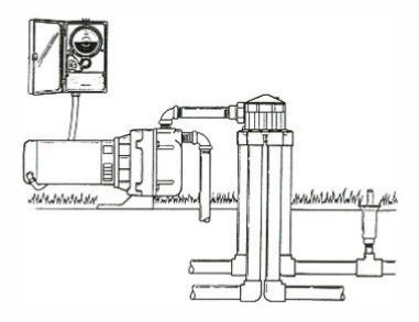
For direct pump - fed installations, the Valve is directly connected to the discharge side of the pump and is cycled from one zone to the next by turning the pump off and on . Install the valve as close to the pump as possible and ensure suction line to the pump has a proper check valve installed and all joints are completely sealed.
