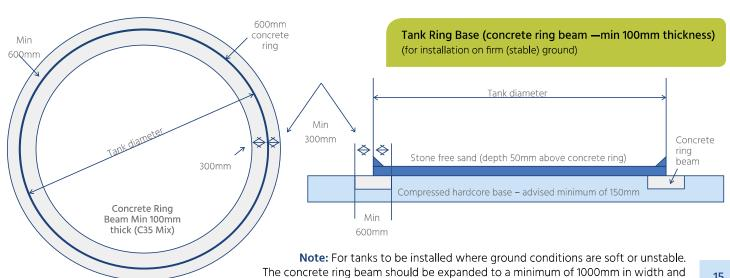
150mm in depth. The hardcore infill may also require an increase in depth to 200mm.
