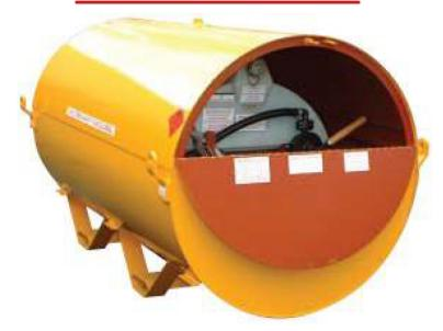
**OUTER BUND TANK:** Constructed from 3mm Mild Steel, cylindrical in section. Removable top section.4 lifting eyes on tank corners. Built-in fork truck sockets in base of tank. Stainless steel Hinged rear access door, fully lockable.
