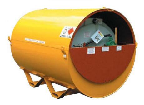
**OUTER BUND TANK:** Cylindrical in section constructed from 3mm mild steel, with removable top section for tank access. Rear access door, fitted with stainless steel hinge and fully lockable. Bund contains 110% of inner tank content. 4 lifting eyes & fork sockets.
