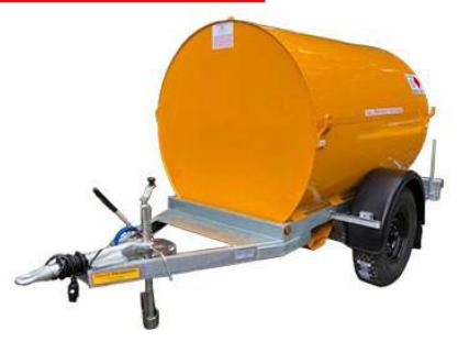
**COUPLING:** 3000kg Knott-Avonride posibrake over run auto reverse c/w spring assisted handbrake lever, breakaway cable. 40mm ring eye or 50mm ball.
