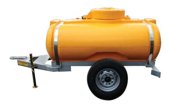
**CHASSIS:** Constructed from 100 x 50 RSC fully welded, with front standing plate and an 'A' frame drawbar, 80x80x6 RSA frame, hot dipped galvanised.
