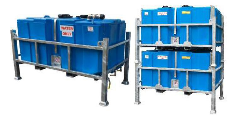
**TANK:** Corrosion free, robust polyethylene Baffled tank, two access lids for easy cleaning, 2" fast drain in base of the tank, two ¾" Valve outlets in the base of the tank, All fittings & lids lockable. Hydrant fill (optional Extra)
