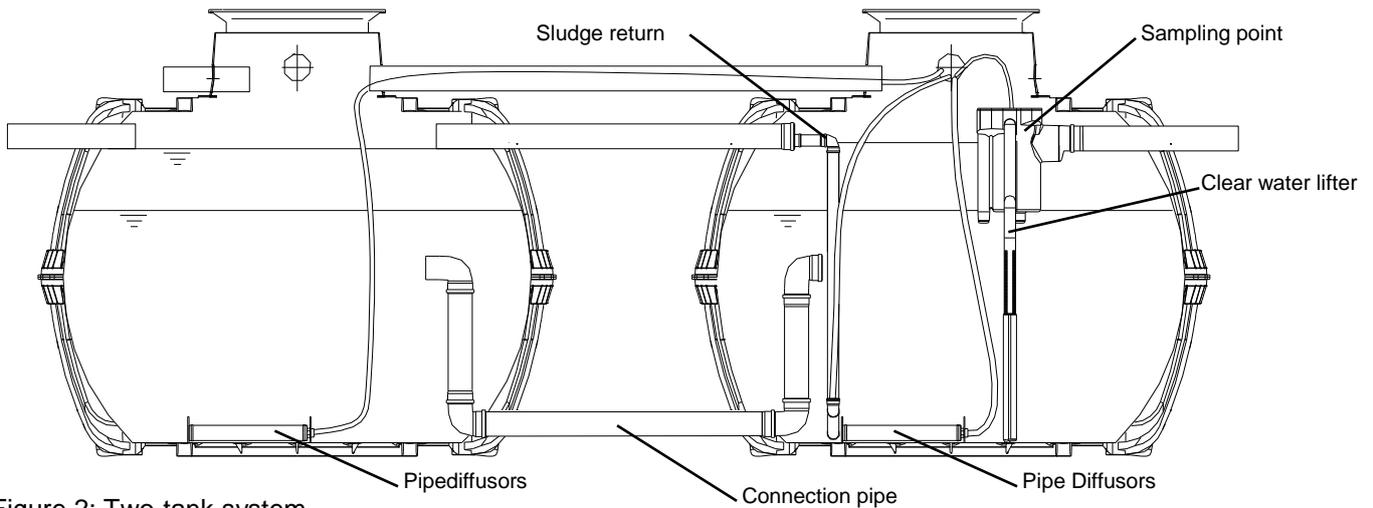
Figure 2: Two-tank system
