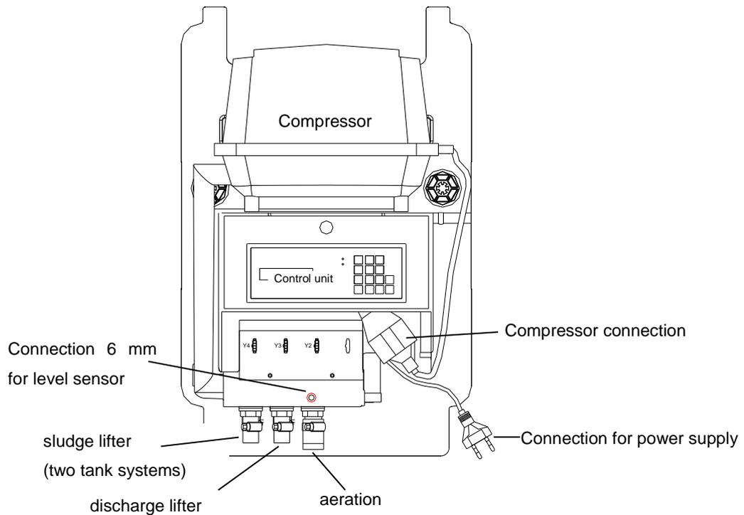
Figure 3: EPP cabinet with 3-way air distributor
