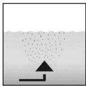
In the first phase, the wastewater is put straight through aerobic treatment for a fixed time. As a result, the microorganisms (aerated sludge) are supplied with the oxygen needed for the breakdown and then pressure aeration causes mixing. The system's aeration equipment is supplied with ambient air by a compressor. Aeration is intermittent so that targeted wastewater cleaning is possible. Different ambient conditions can thereby be achieved.
